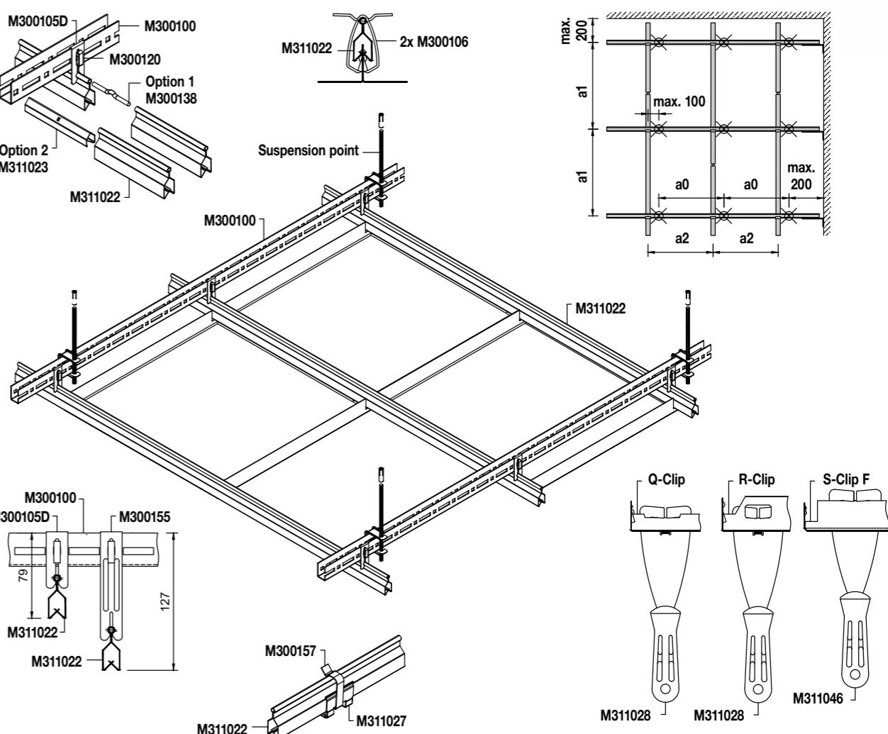
\* System with additional load + 4 kg/m<sup>2</sup>
