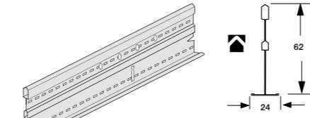
The Prelude 24 Sixty<sup>2</sup> butt cut system is designed for use in corridor applications, with or without Cross Tees, and where spans do not exceed 3750 mm.
