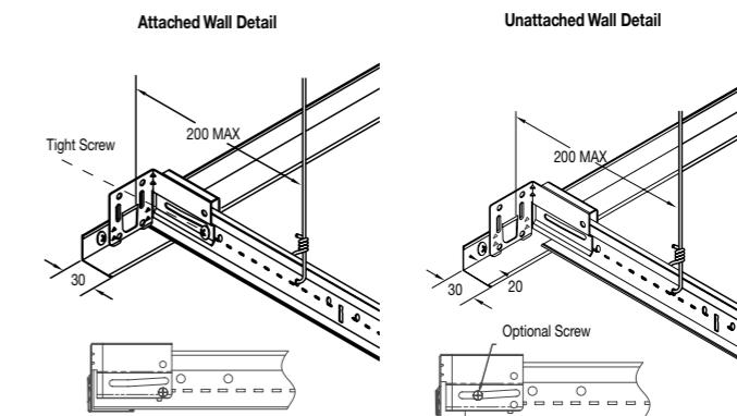
The Seismic Rx® system installation method will depend upon the hazard level required for the installation.
